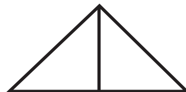
Fig. 2: King Post Truss
